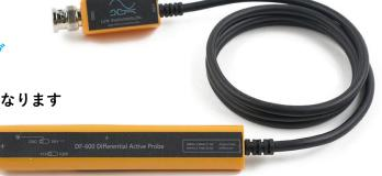
A lot of money will be spent if both a differential probe and an active probe are needed. If a conventional differential probe is used as an active probe, there will be a big problem when there is a big voltage difference between the target ground and the oscilloscope ground. This DF-600 Differential Active Probe has a switch to select differential or single-ended mode and another switch to change the measured voltage range.
