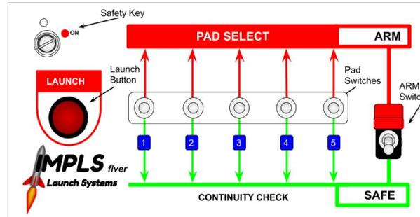
You will now test remote continuity to make sure that everything is ready for use. Insert the Safety Key and rotate to the ON position. The ARM switch should be SAFE and the paddle down to indicate Safe. Toggle Pad Switches 1-5 according to which launch leads you shorted at the controller. If they beep then you are ready for operation. Remote continuity check will only work when Console is Safe.
